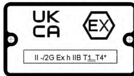
Figure 14: Typical UKCA Ex nameplate
