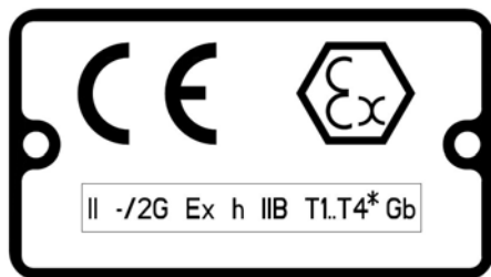
Figure 13: Typical Ex nameplate
