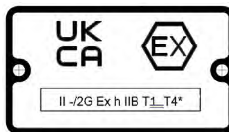
Figure 2: Typical UKCA Ex nameplate
