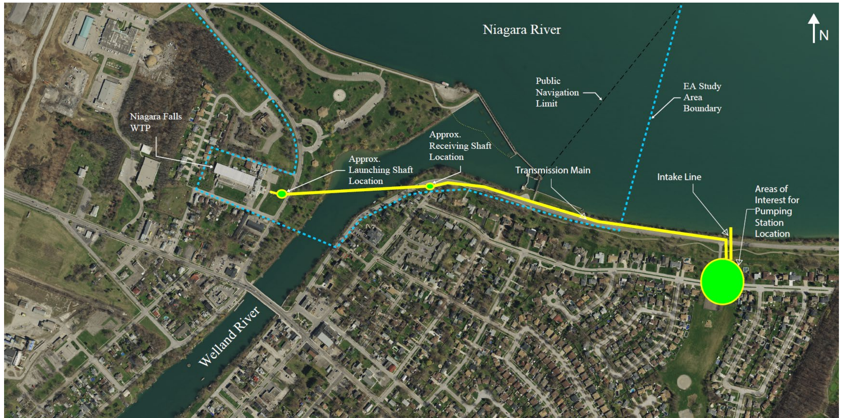
Figure 5.2-1 Niagara Falls WTP - Raw Intake Relocation – Alternative 2A Preferred Design Concept
