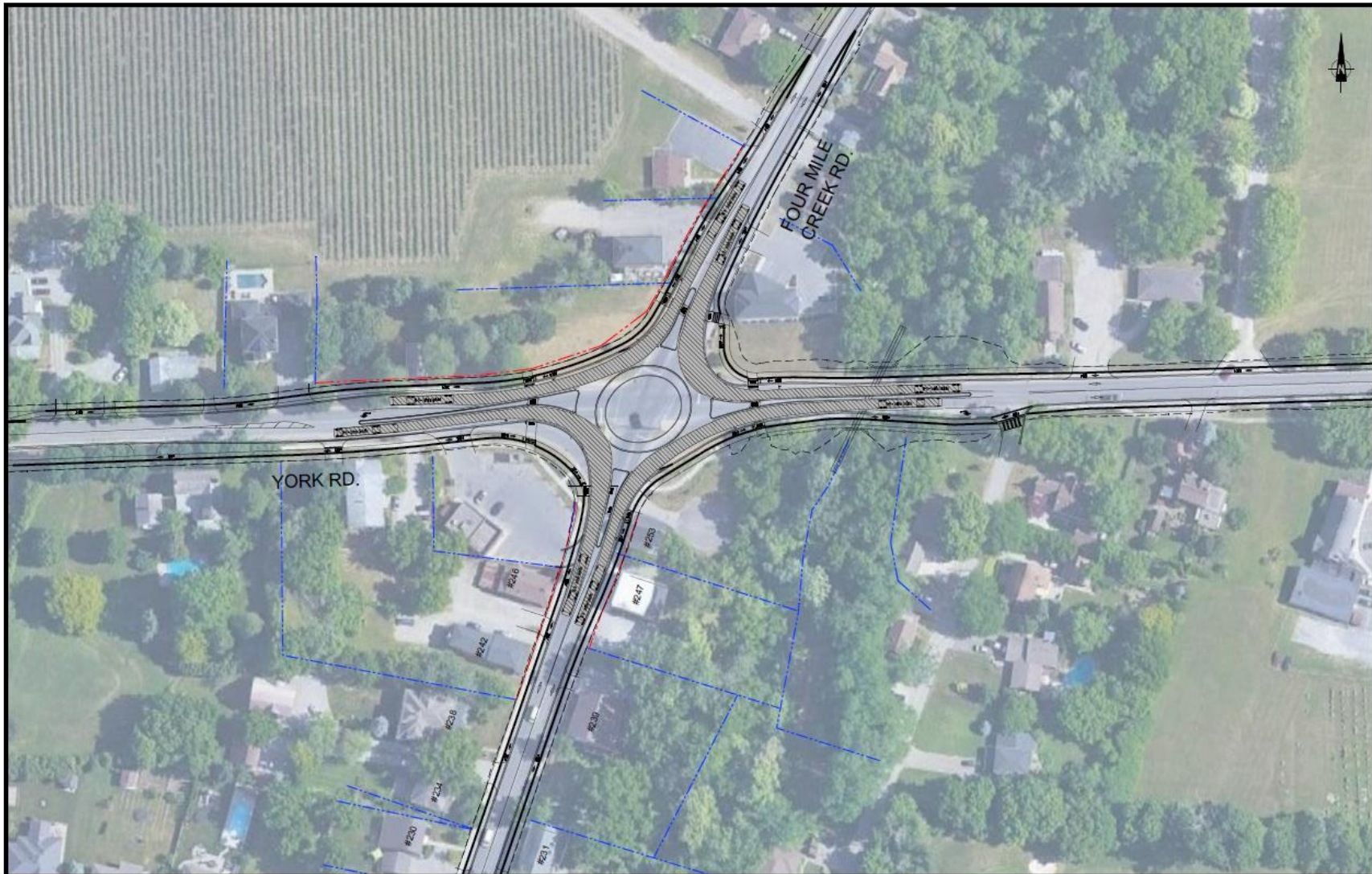
Figure 6-24: Roundabout Design – Vehicle Right Turns
