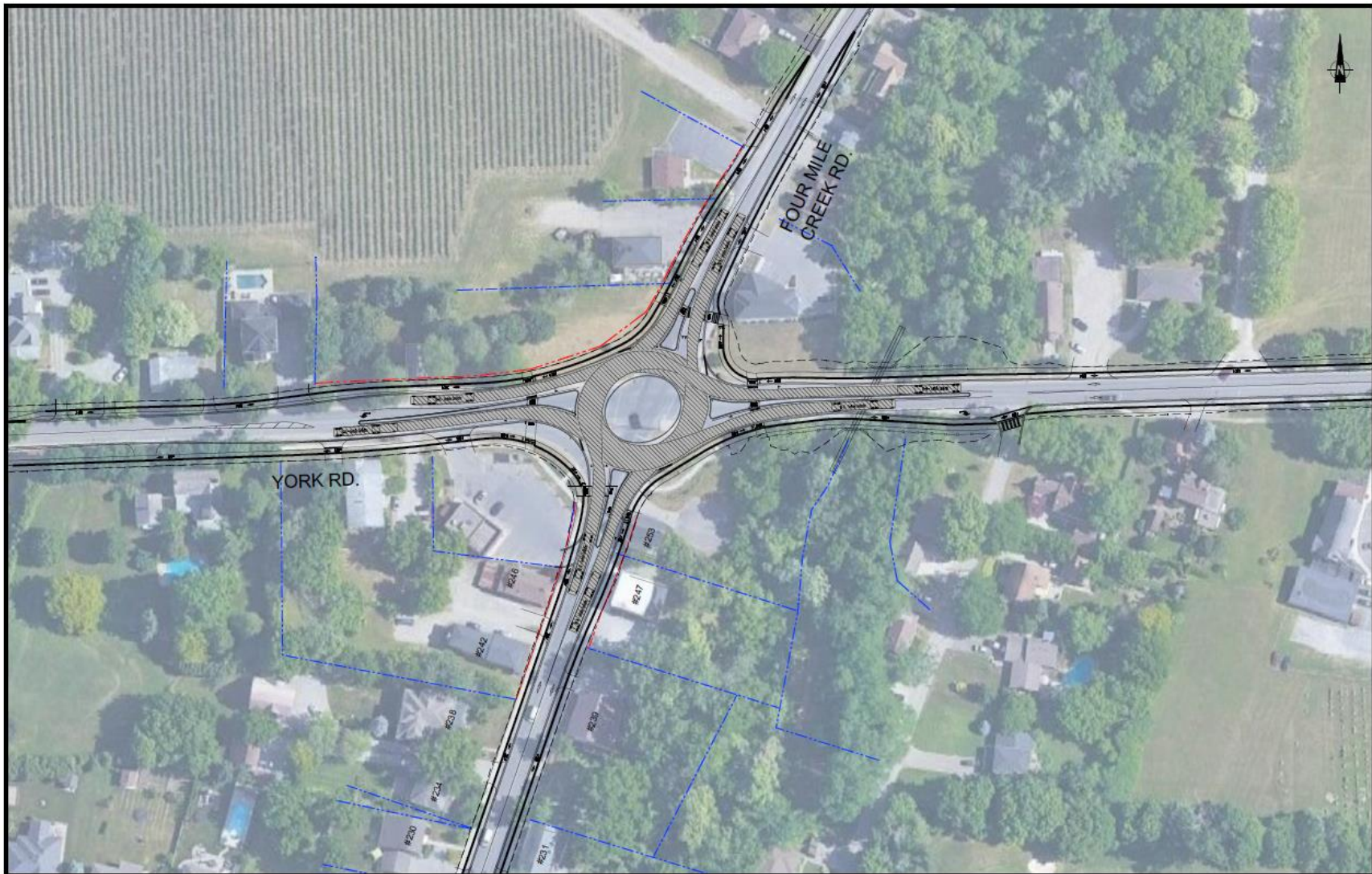
Figure 6-23: Roundabout Design – Vehicle Left Turns
