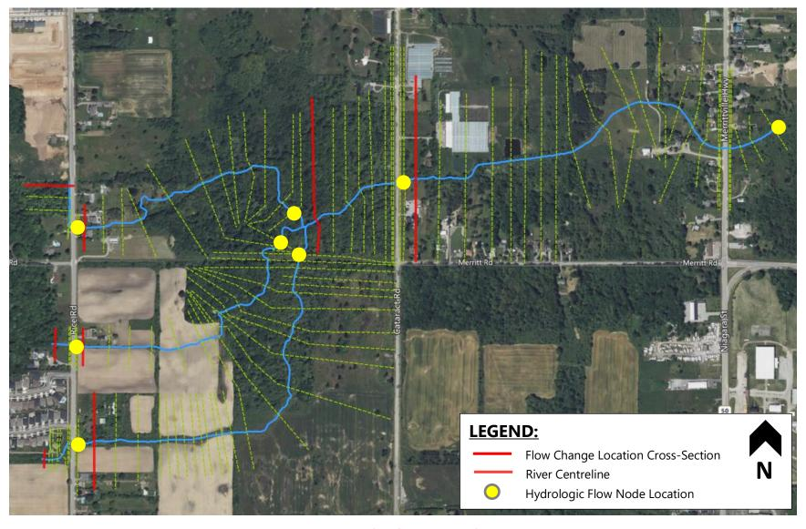
Figure 4-4: Flow Change Location Plan
