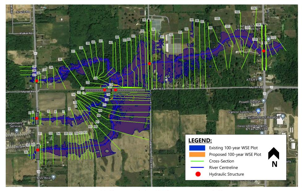
Figure 4-6: Proposed Floodplain 100-year Hydraulic Model Results – Comparison to Existing Floodplain
