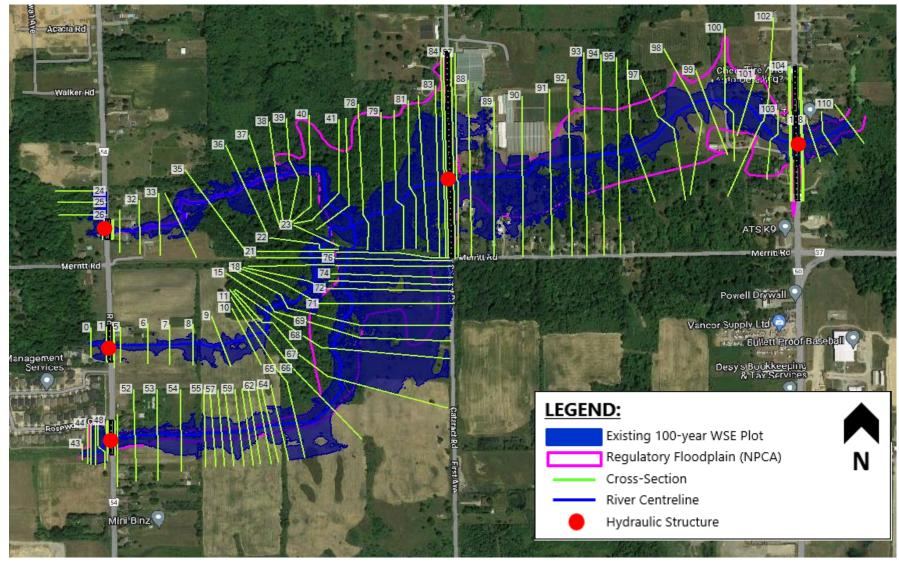
Figure 4-5: Baseline 100-year Hydraulic Model Results – Comparison to Existing Regulatory Floodplain
