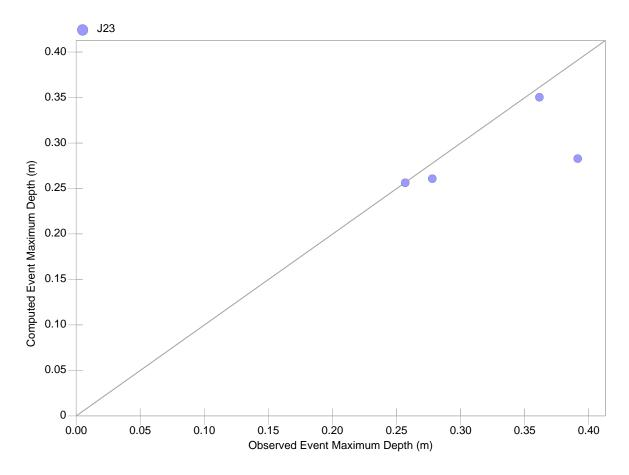
Figure 3-6: Scatter Plot of the Observed and Simulated Maximum Flow Depths (m) of Rice North Station (J23)
