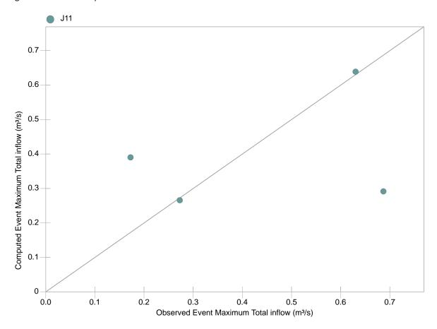
Figure 3-3: Scatter Plot of the Observed and Simulated Peak Flows (m<sup>3</sup>/s) of Rice South Station (J11)
