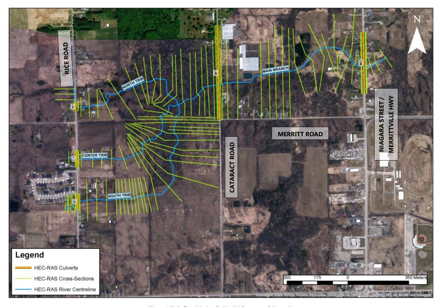
Figure 4-2: Refined Hydraulic Model Geometry Schematic
