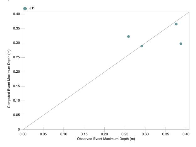
Figure 3-5: Scatter Plot of the Observed and Simulated Maximum Flow Depths (m) of Rice South Station (J11)
