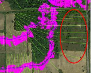
Figure 4-3: Example of "No Levees" Scenario vs. "with Levees" Scenario (a – on the left side): Example of "No Levees" Scenario – No simulated flow within the main channel due to other low points within the floodplain.
