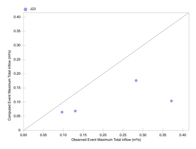
Figure 3-4: Scatter Plot of the Observed and Simulated Peak Flows (m³/s) of Rice North (J23)
