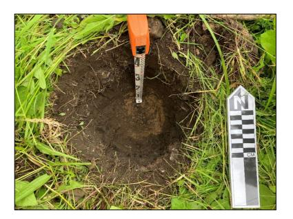
Example test pit showing the soil profile of brown clay loam over buff brown subsoil.
