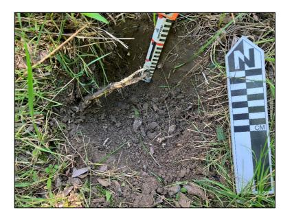
Example of a test pit showing evidence of land disturbance. A brown sandy loam overlays a layers of gravel screenings.
