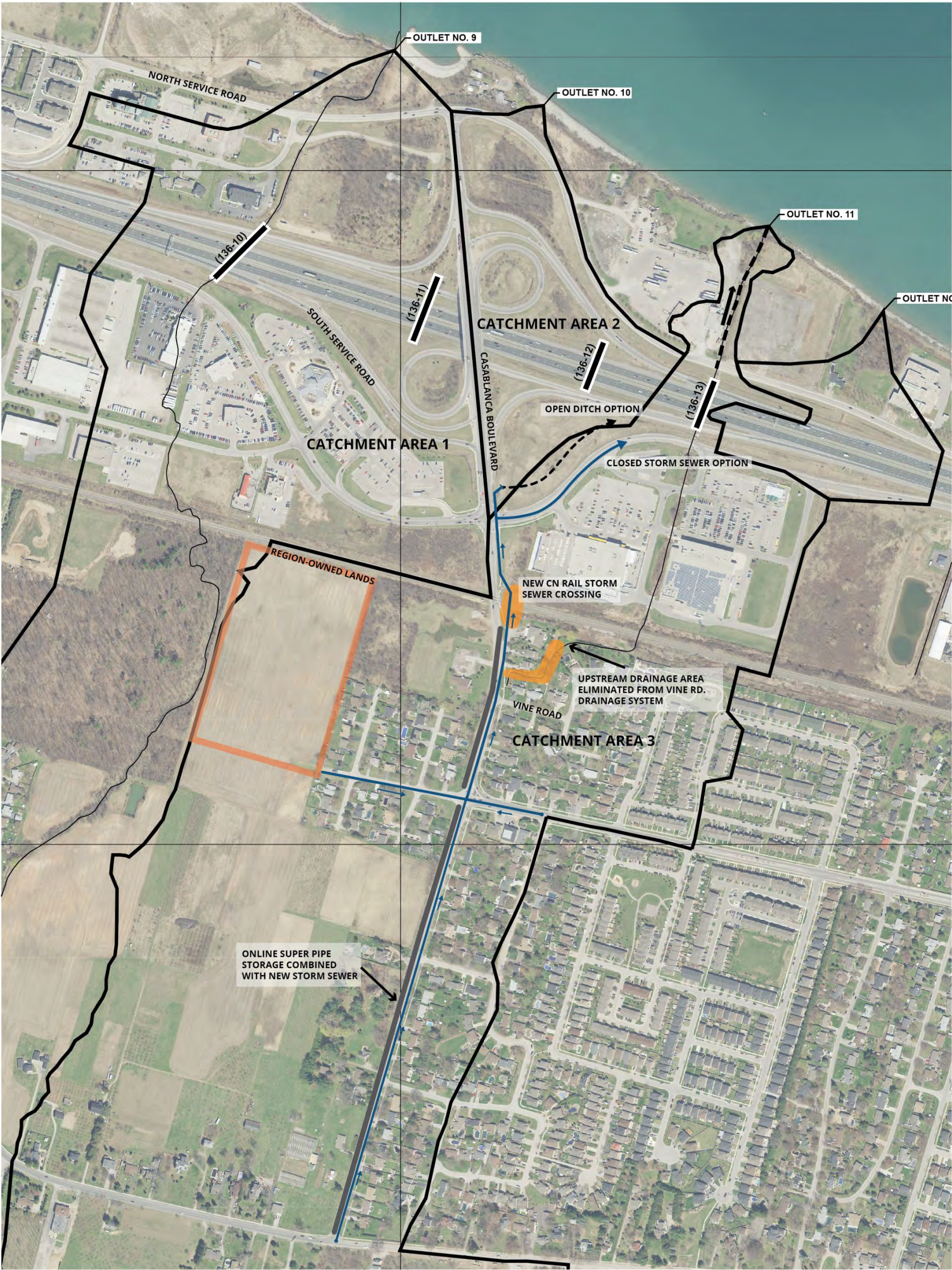
Figure 7-14 Stormwater Management Alternative D - New Conveyance with Super-Pipes and New Storm Sewer Outlet
