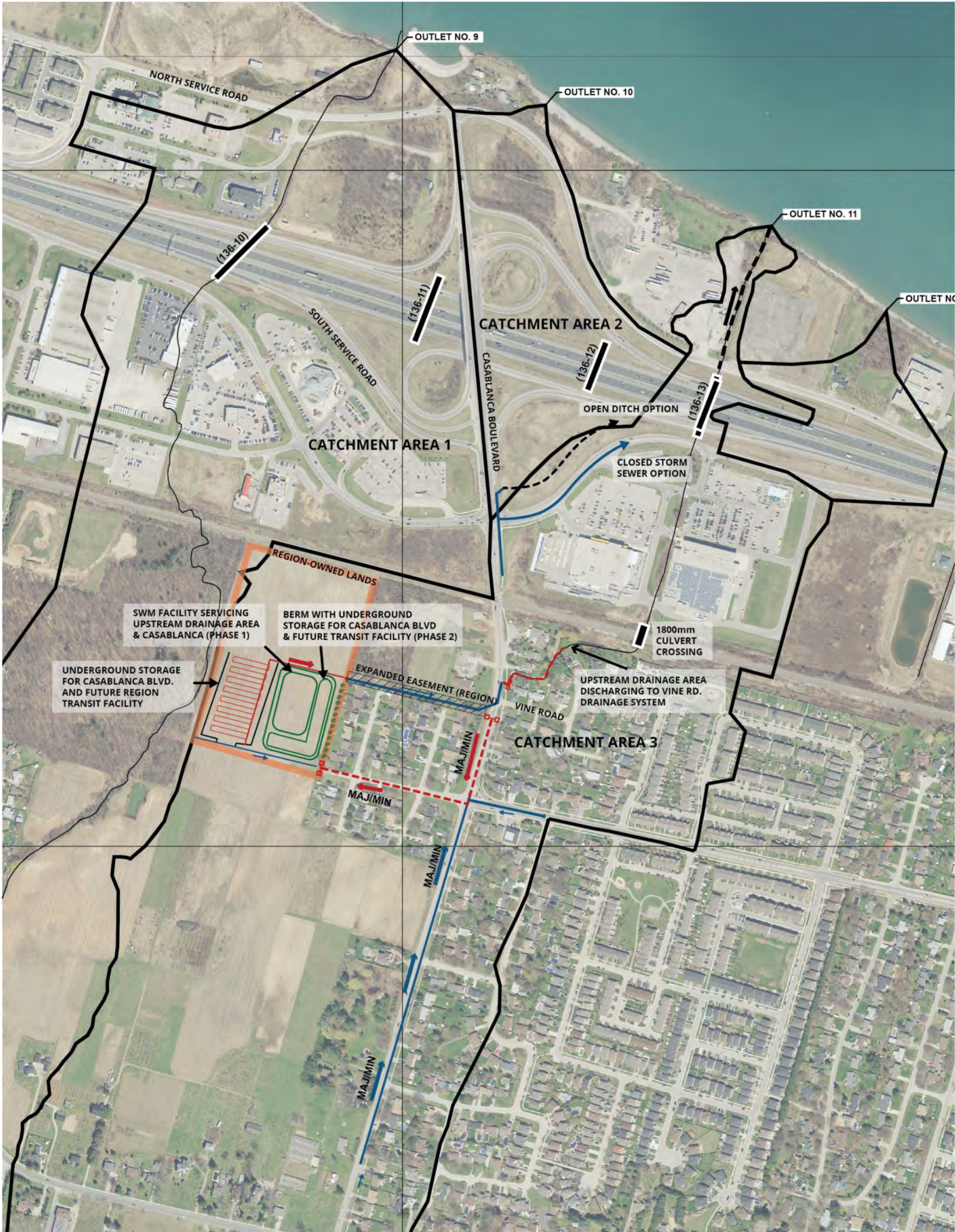
Figure 7-12 Stormwater Management Alternative B - New Conveyance, End of Pipe Control and Use of Vine Road Drain
