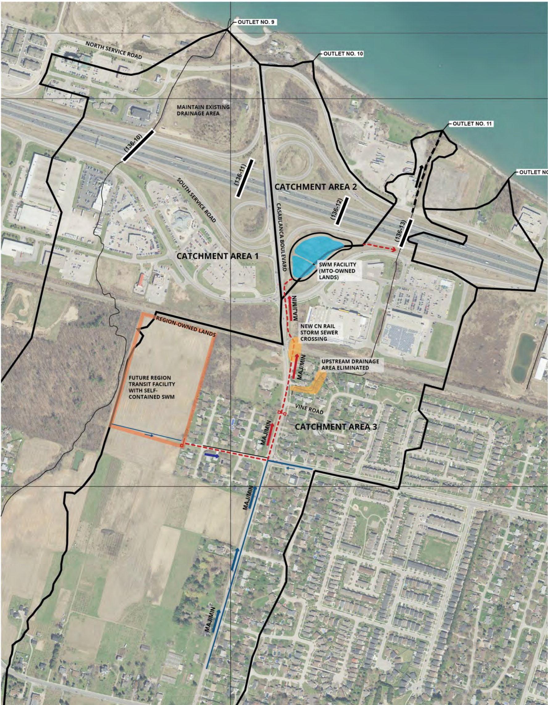
Figure 7-11 Stormwater Management Alternative A - Conveyance and End of Pipe Control in MTO Corridor
