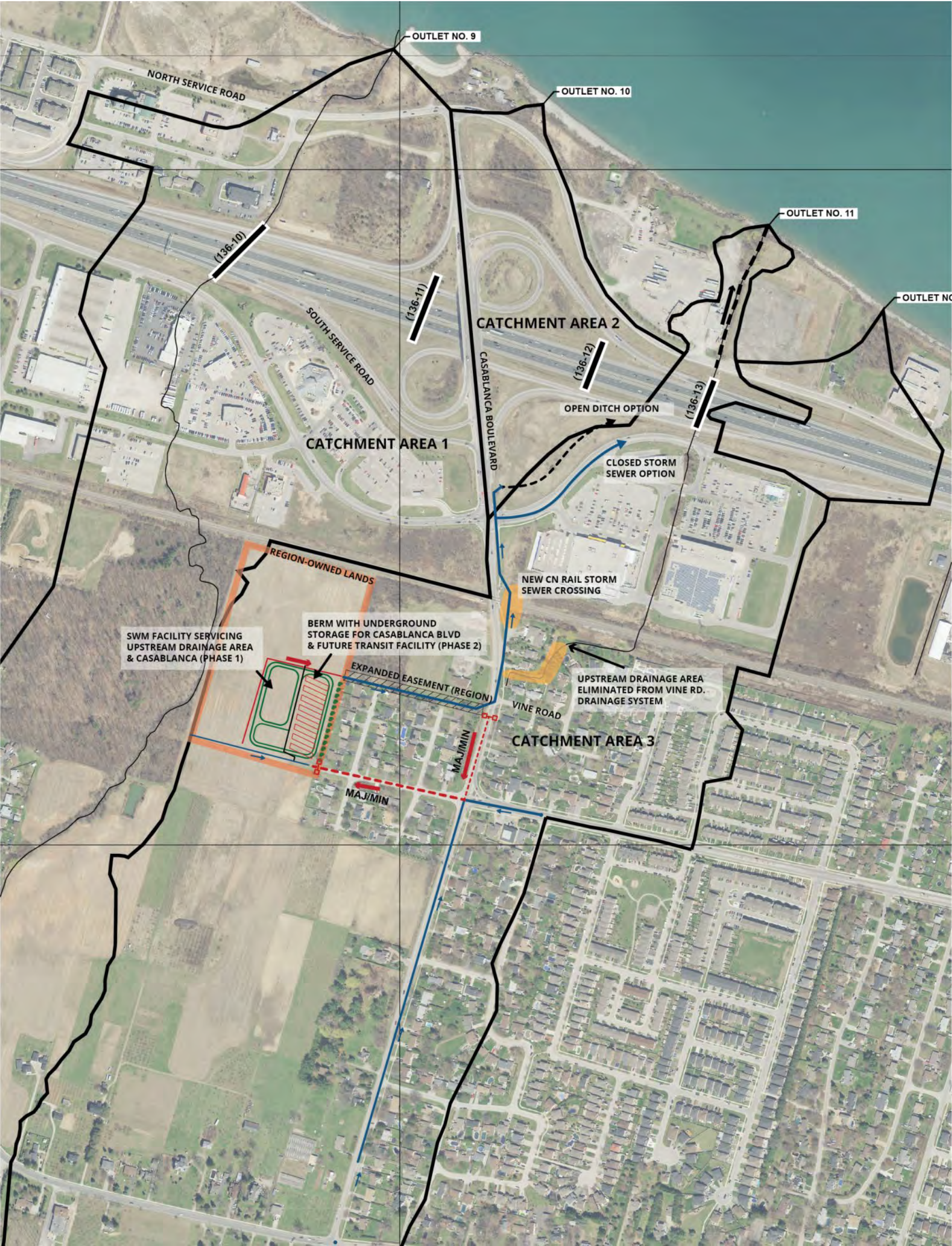
Figure 7-13 Stormwater Management Alternative C - New Conveyance and End of Pipe Control
