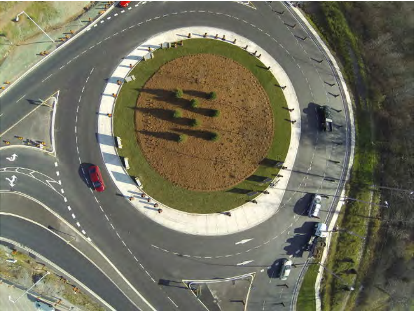
Roundabouts, such as this example at East Main Street in Welland, may reduce traffic delays and queues (Credit: Welland Tribune: http://www.wellandtribune.ca/2014/09/05/at-least-five-crashes-since-roundabout-opened ).
