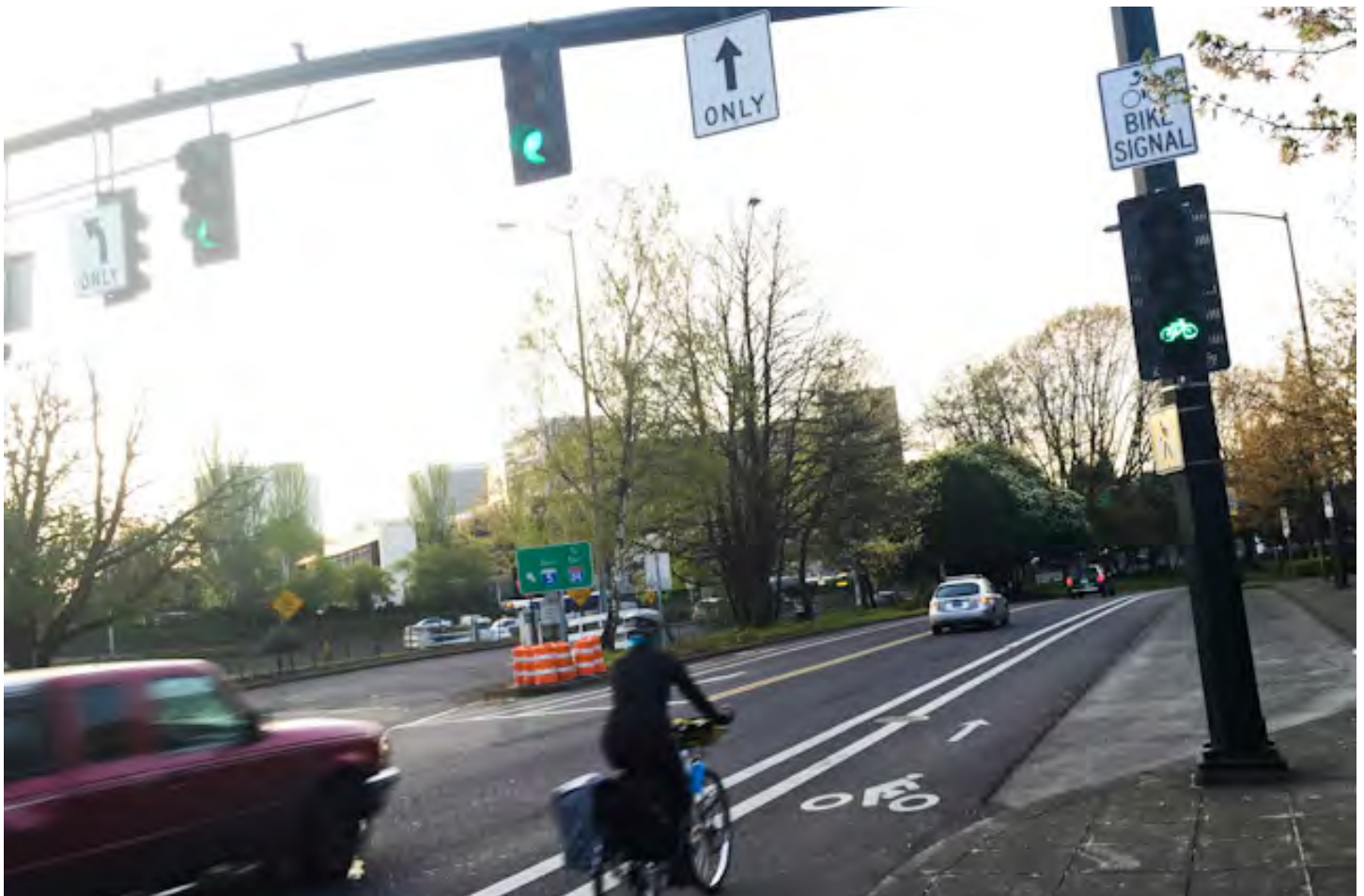
Bicycle Signal in Portland, OR provides green light for cyclists (Credit: BikePortland.Org: http://bikeportland.org/2015/04/13/new-bike-signal-north-moda-center-adds-greentime-southbound-biking-139306 ).
