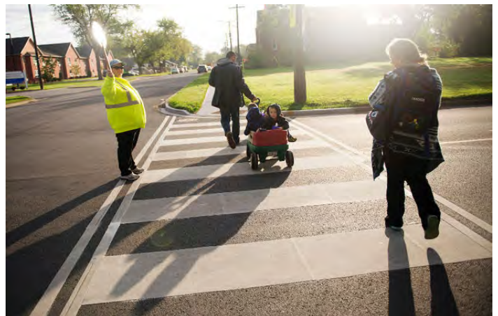
Zebra markings such as these shown at the intersection of Plymouth Road and First Street in Welland improve crosswalk visibility and pedestrian safety
