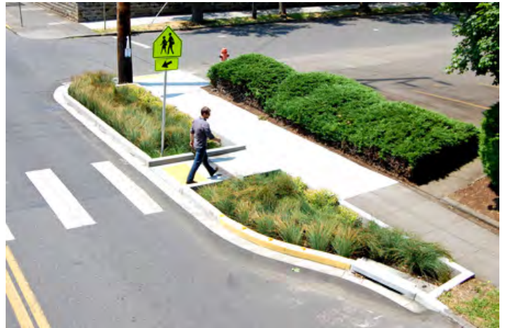
Curb extensions at intersections minimize the crossing distance for pedestrians while increasing the available space for vegetation and street furniture.
