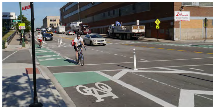
Intersection Crossing Markings - Chicago, IL (Credit: NACTO: http://nacto.org/publication/urban-bikeway-design-guide/intersection-treatments/intersection-crossing-markings/ ).
