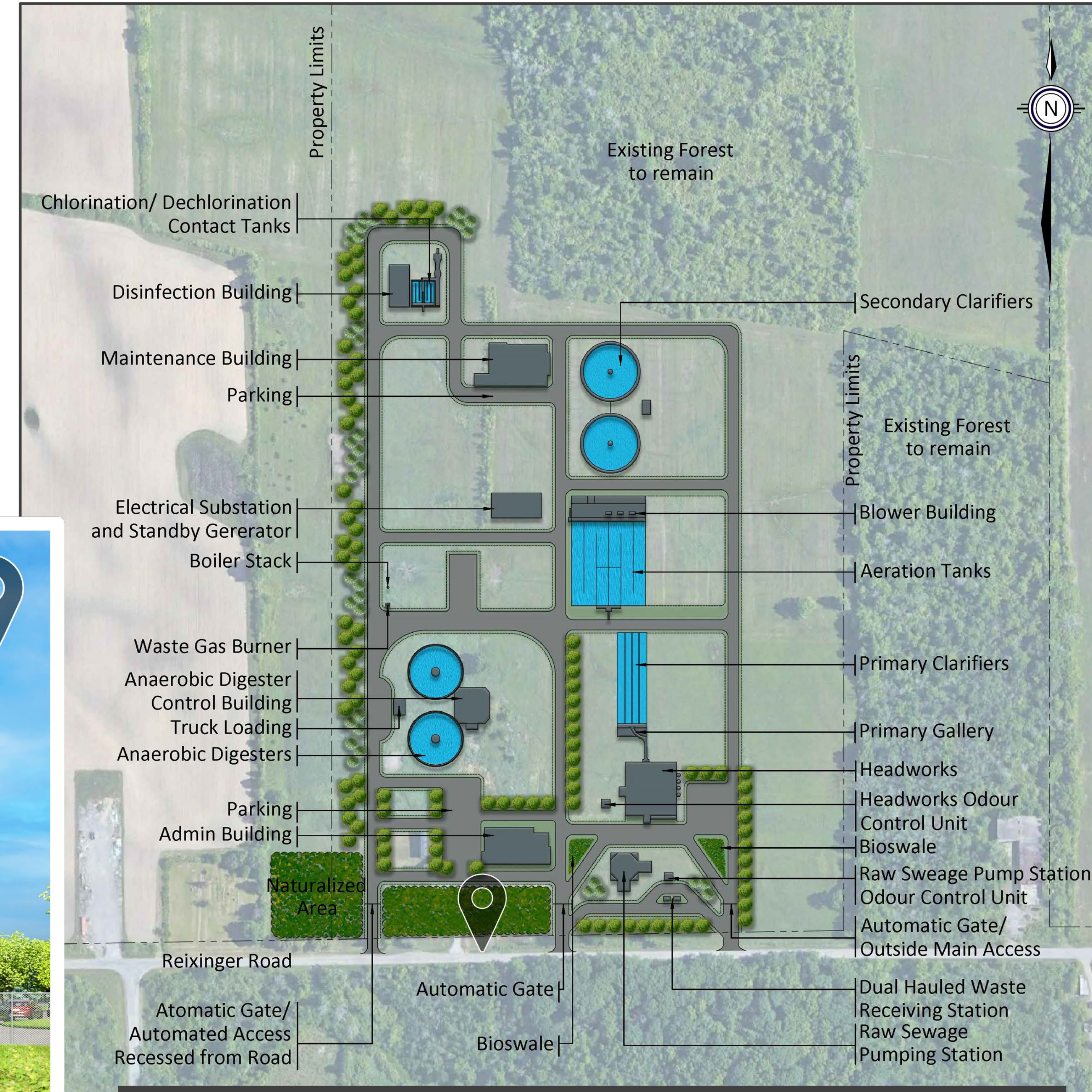
Preferred WWTP Layout (6811 Reixinger Road)
