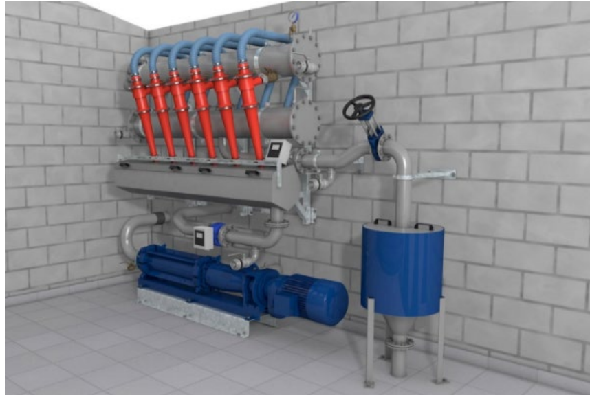
Figure 9 Select® Hydrocyclones and Recycle System (ETA)
