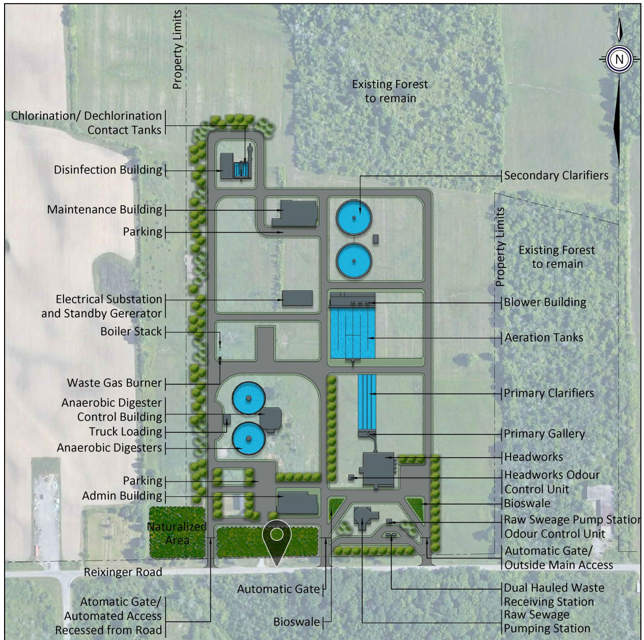
Figure 7-1. Preferred WWTP Design Components
