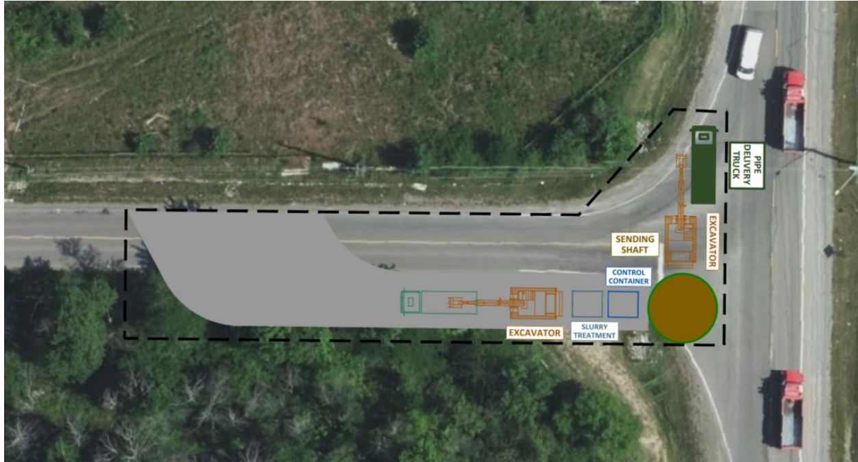
Figure 6-4. Example Launch and Sending Shaft
