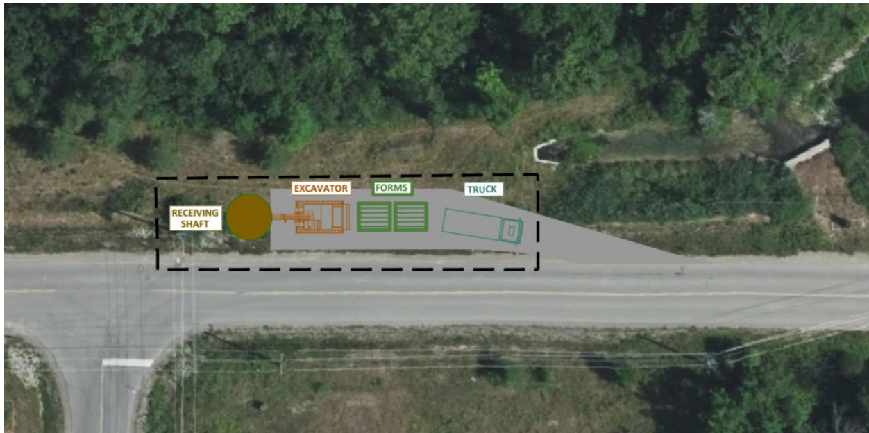
Figure 6-5. Example Receiving Shaft
