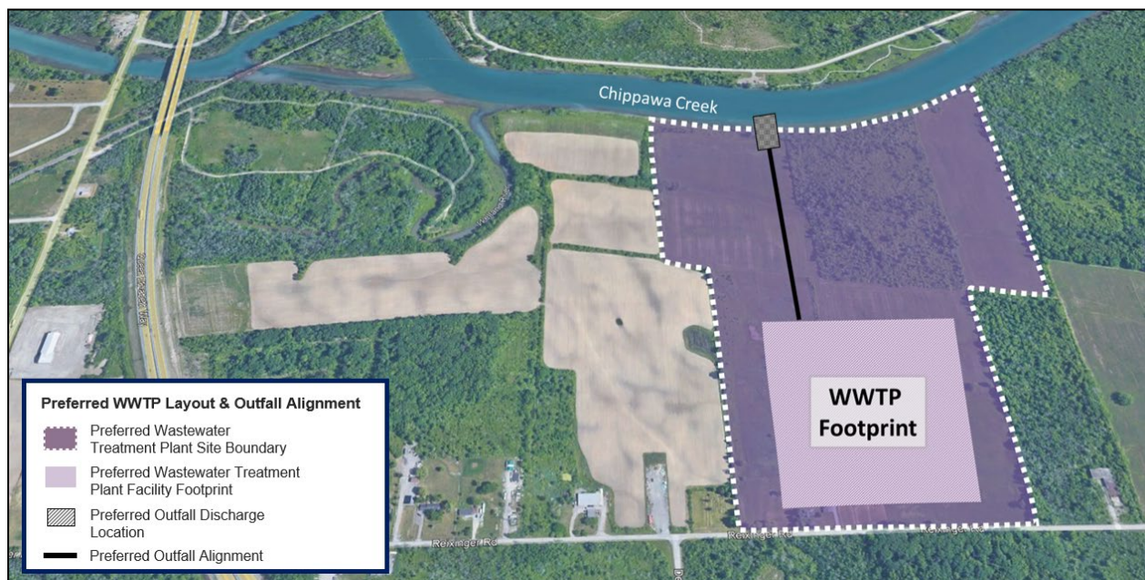
Figure 6-2. Preferred WWTP Site Layout and Outfall Alignment
