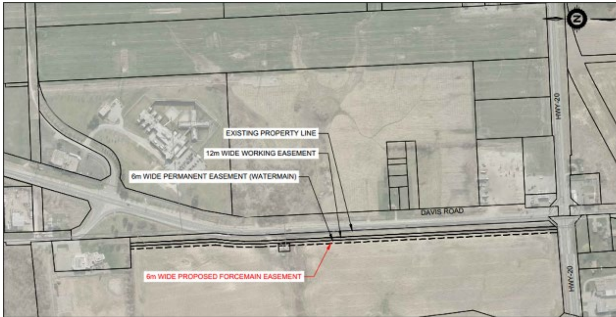
Figure 9-1. Proposed Forcemain Easement from New Black Horse SPS Site to Highway 20
