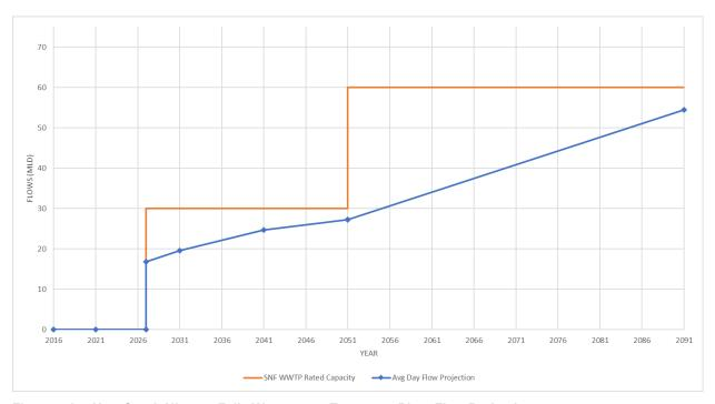
Figure 5-2. New South Niagara Falls Wastewater Treatment Plant Flow Projections
