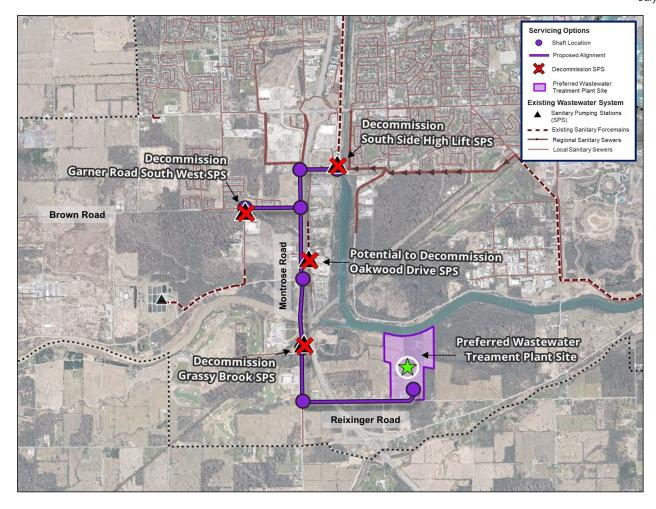
Figure 6-4. Preferred South Niagara Falls Trunk Sewer Alignment
