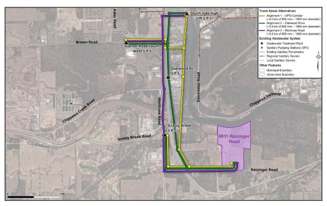
Figure 5-6. New SNF Trunk Sewer Alternatives
